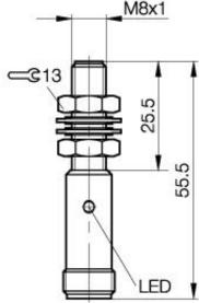
**Inductive Sensors** BES 516-324-E5-C-S 4 M8x1 x 55.5 normally-open **Sn=1,5mm** shielded
